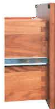
¾" Hardwood dovetail drawer boxes with ½" bottoms standard on all cabinets.
